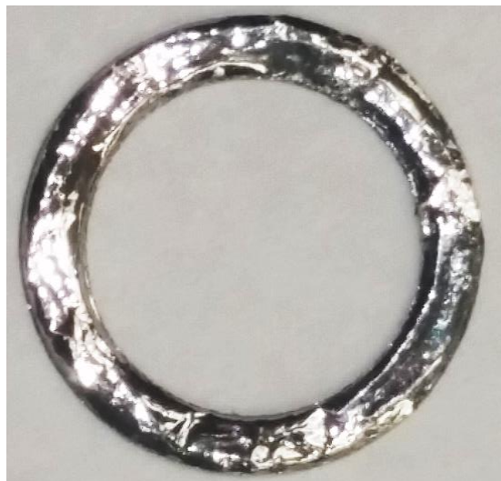
Figure 4.22. New high frequency magnetic material from 3M.
