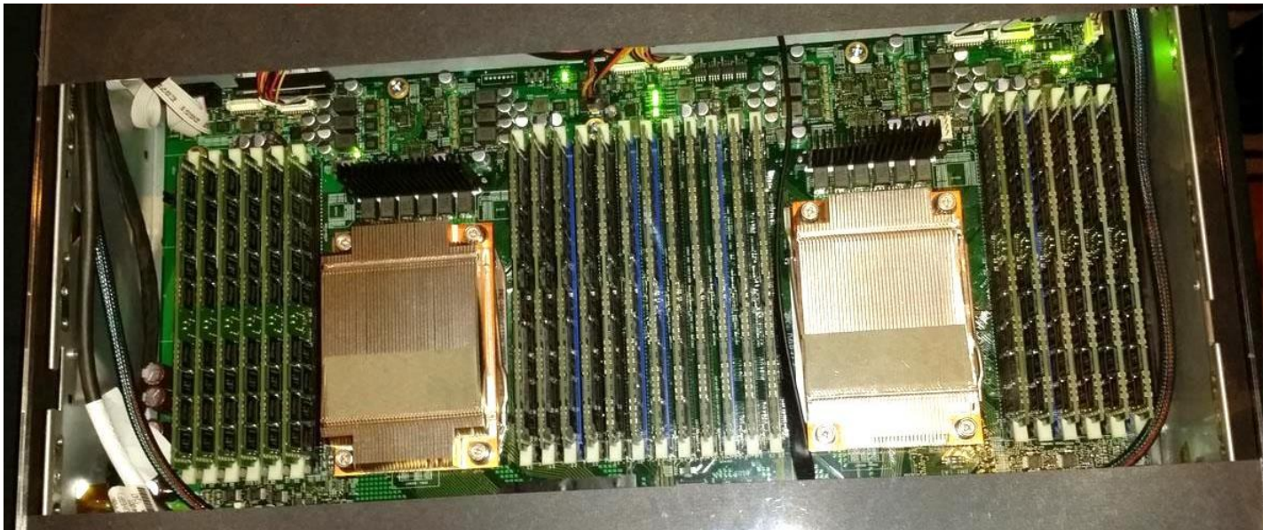
Figure 2.9. Intel’s two-processor, one-unit (2P 1U) server platform.
