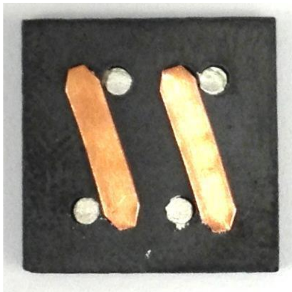
Figure 1.16. Fabricated lateral flux coupled inductor substrate for 4 MHz POL module.
