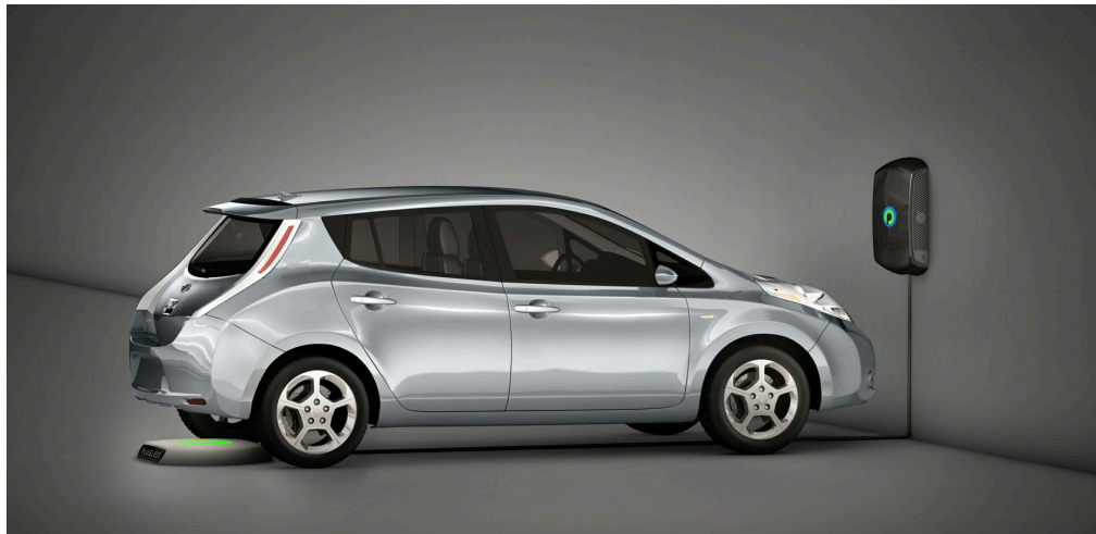
Fig. 1.7. Nissan Leaf EV charged by a wireless battery charger [4].
