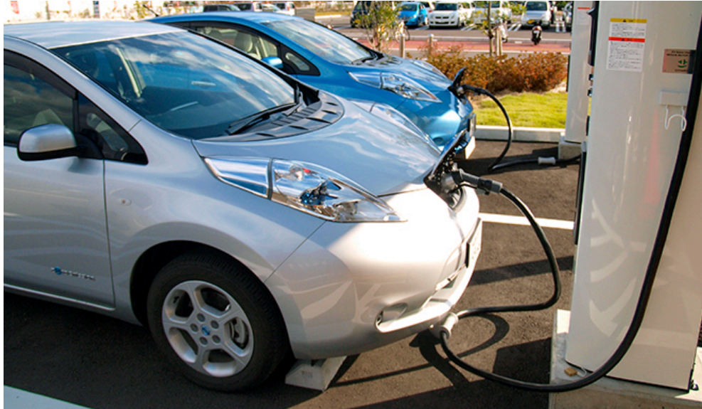
Fig. 1.6. Nissan Leaf charged by a conductive battery charger [4].
