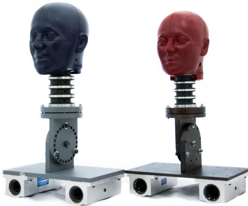
Figure 1: The adult surrogate (left) features a blue NOCSAE headform, 50 th percentile Hybrid III neck, and 16 kg steel sliding mass. The youth surrogate (right) was scaled to include a red NOCSAE headform, 5 th percentile Hybrid III neck, and 8 kg aluminum sliding mass.
