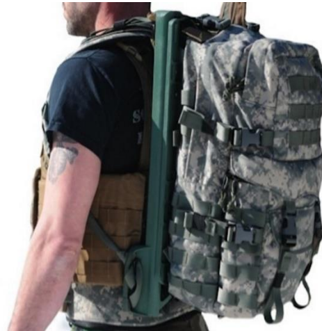
Figure 2-8 Current backpack energy harvesting application for soldiers: (a) Energy Harvesting Assault Pack (EHAP) [30]; (b) Lightning Packs [31].
