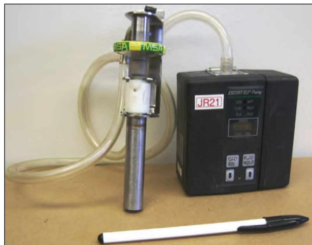
Figure 24: Personal dust sampler - Escort EFL pump with cyclone and filter (J Colinet et al., 2010)
