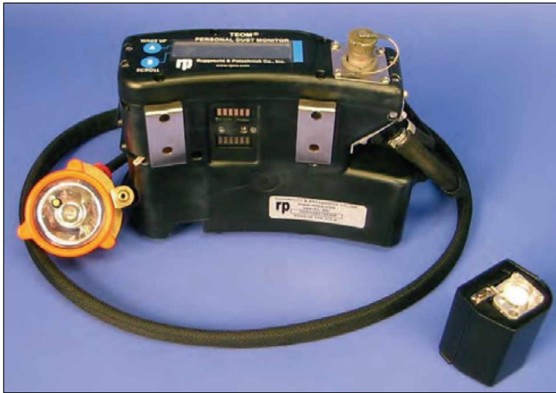
Figure 23:CPDM with filter casing removed (J Colinet et al., 2010)
