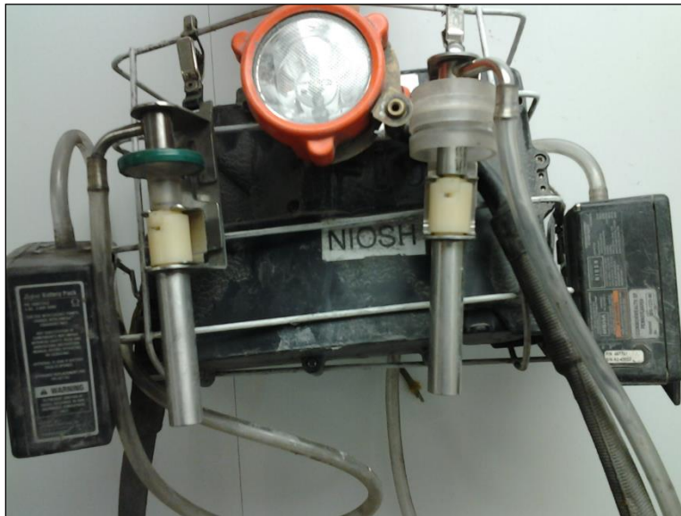
Figure 25: Example of equipment setup utilizing a CPDM and two personal dust samplers
