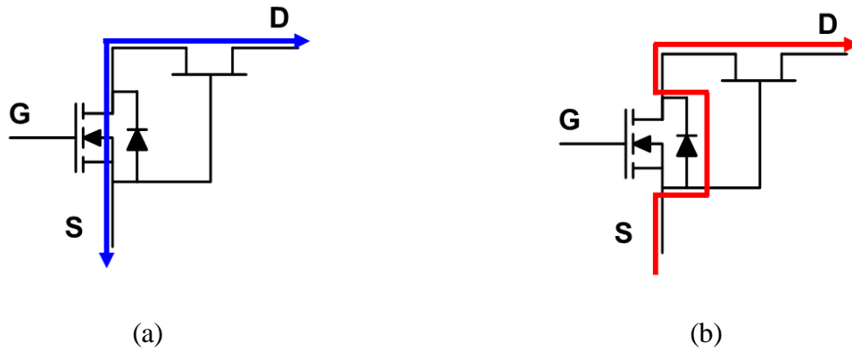
Fig. 1.9. Conduction principle of cascode GaN HEMT, (a) V_{gs}=10V , (b) V_{gs}=0V
