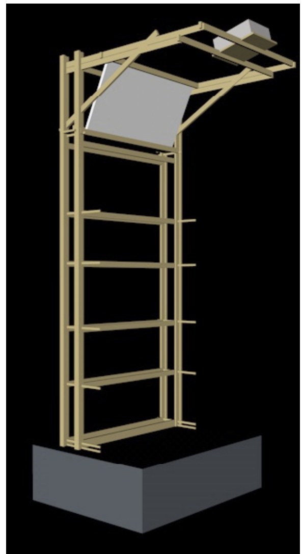
9.7 Proposed rig to be built to achieved the desired projection size. Hight should be at least 25ft high
