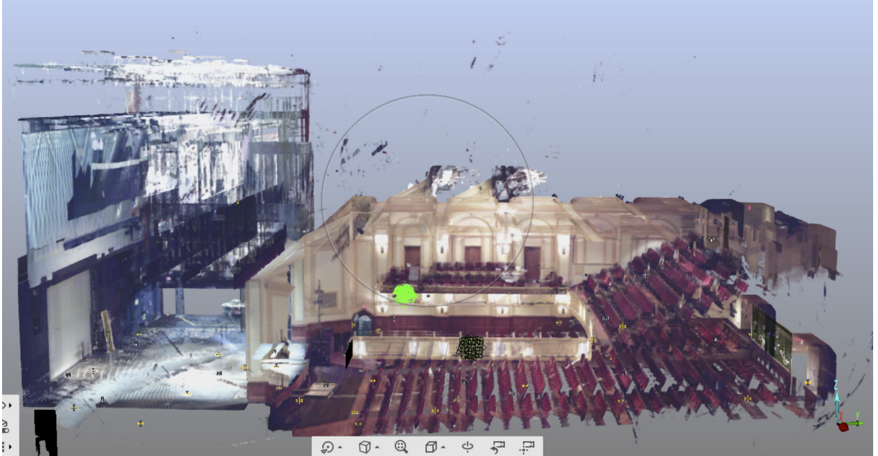
9.1 Jefferson Center Shaftman Performance Hall, 3D Laser Scan and Side Cut Away View
