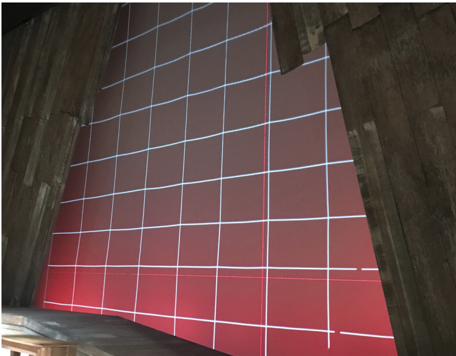
11.6 After the correction, grid is pretty much flat without distortion
