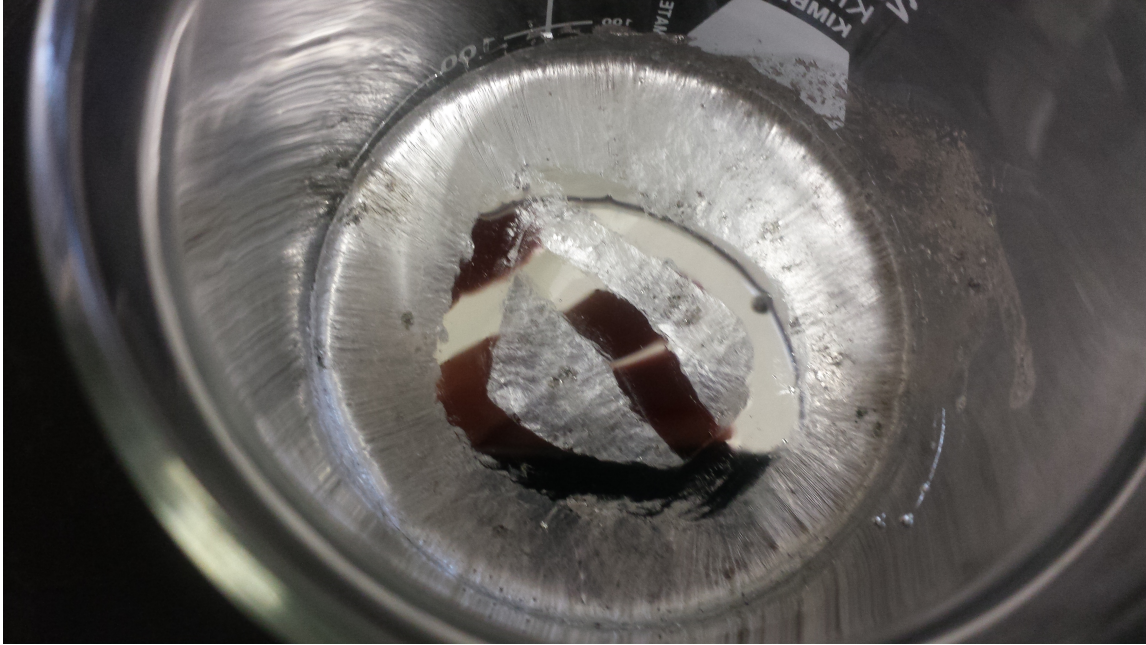
Figure 2.2: Broken Oxidation Layer from Agitation
