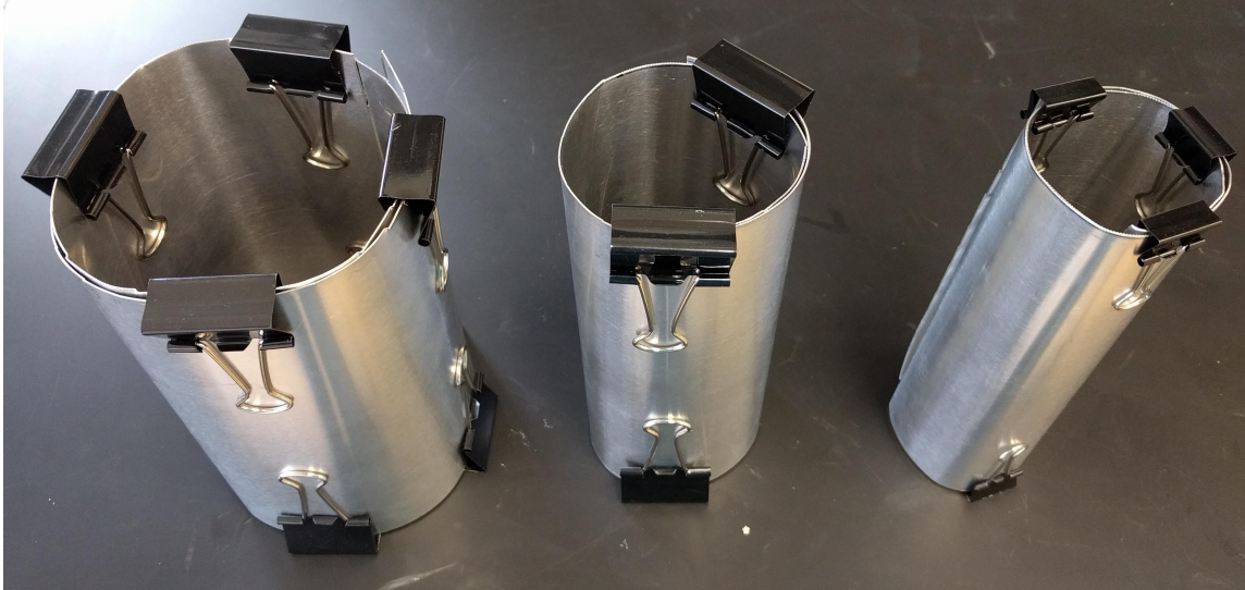
Figure 3.41: Prototype Wheeler Caps (From Left to Right: 1 GHz, 1.5 GHz, 2 GHz)
