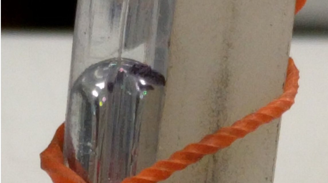
Figure 3.4: Meniscus at EGaIn/NaOH Boundary
