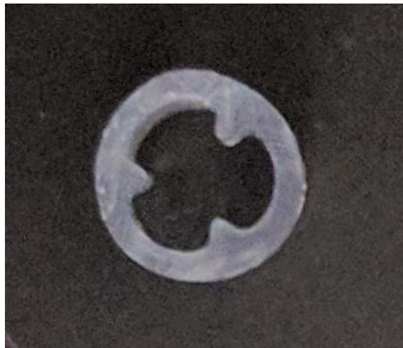
Figure 3.22: Ridges Along the Inside of the Tubing Possibly Cause Oscillations in the Return Loss at High Frequencies
