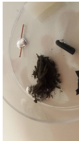
(b) Aluminum Wire Fully Corroded
