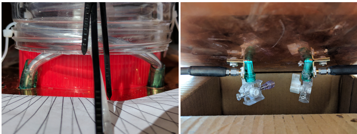
(c) Helix Raised Using Jar Cap to Prevent Tubing from Pinching
