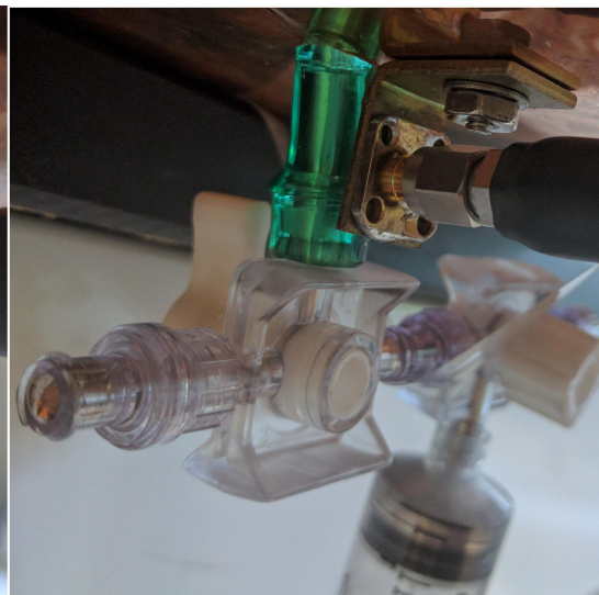
(b) Bottom-Fed Monopole Antenna with Injection Stub
