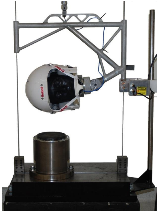
Figure 6. A NOCSAE style drop tower was used to quantify the performance of each helmet.
