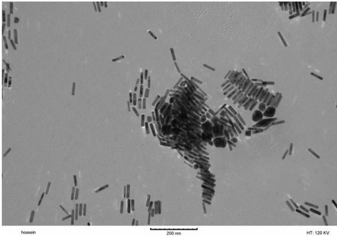
Figure 3.8 TEM image of synthesized gold nanorods using two-step technique
