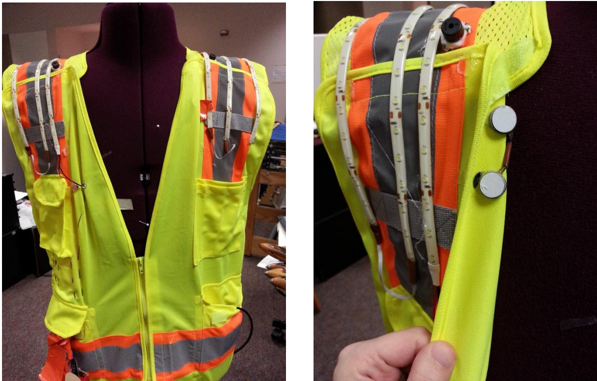
Figure 3.4. The vest used for the second set of studies. The left picture shows the vest, while the right picture shows each of the modalities.
