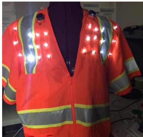
Figure 3.3. Finalized vest created for preliminary studies. This vest was used for initial and preliminary tests, which informed the design for the second construction vest.
