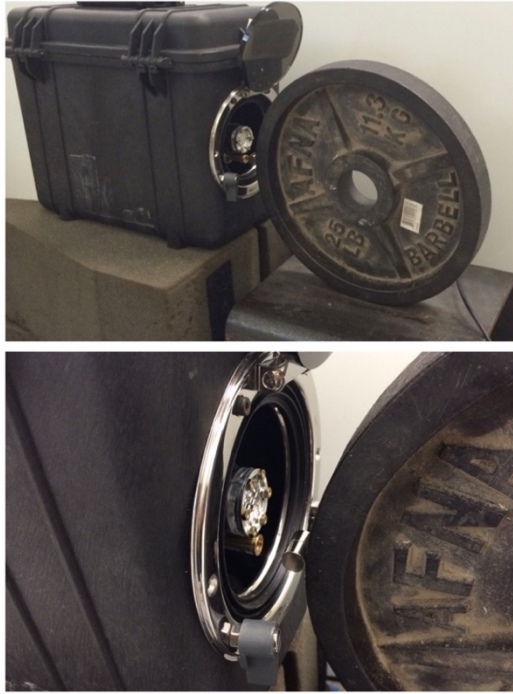
Figure 3-9: One of the experimental setups. Microphone at the radial location and the defect at 0 degrees
