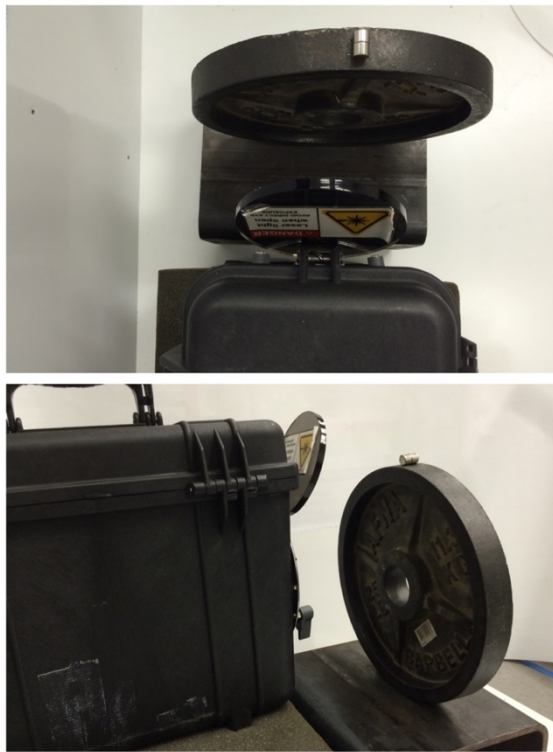
Figure 3-10: One of the experimental setups. Microphone at the axial location and the defect at 90 degrees
