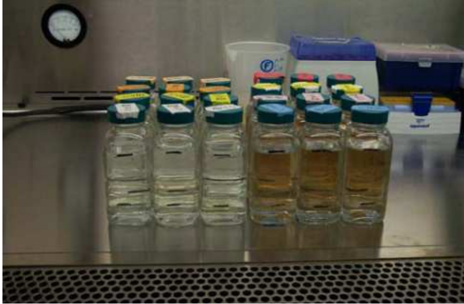
Figure 2: Experimental SGWH Setup; 24 SGWH run in triplicate with TOC concentration from 0-30,000 \mu\text{g/L} . Full SGWH volume (100mL) was changed (80mL was poured out) and refilled 3 times per week to simulate a low-use water system.
