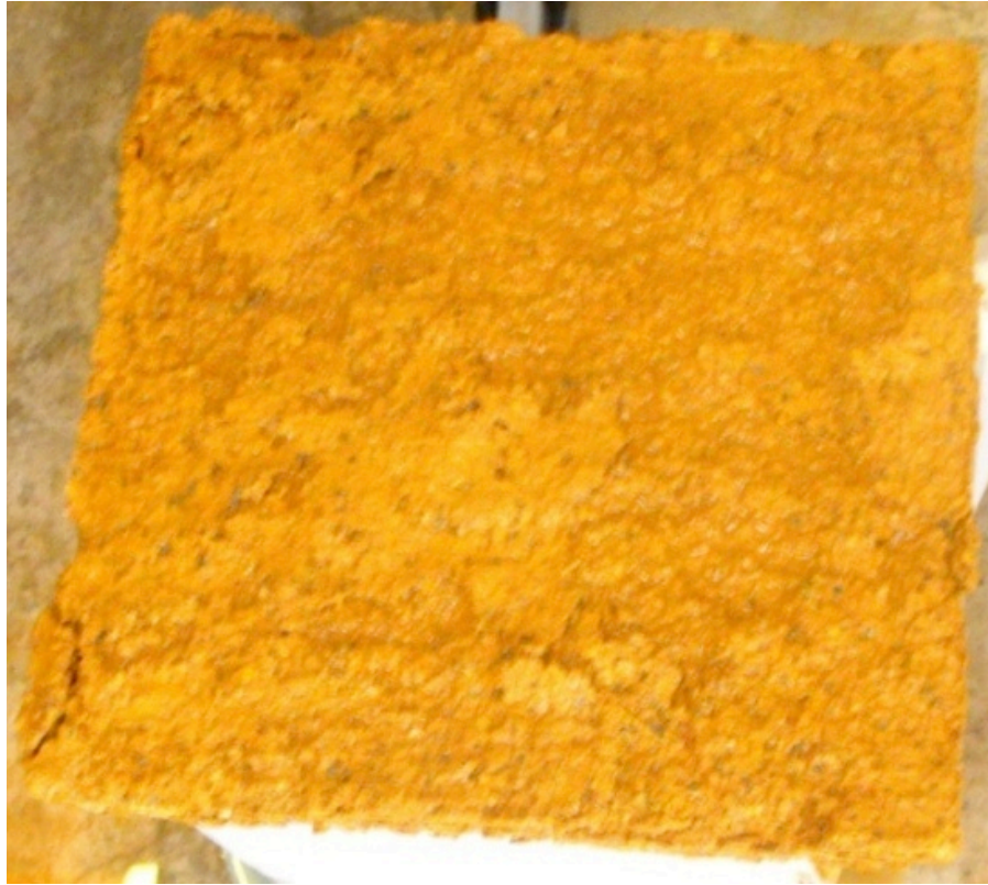
Figure 5.18: Image of result of weight test Panel-3 Earth + Elmer's glue, disintegrated fragment after ½ hour
