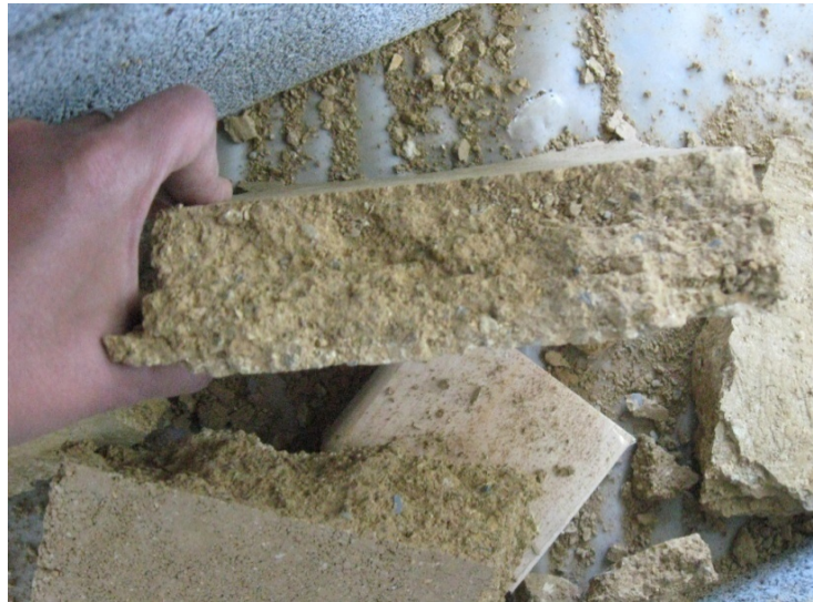
Figure 5.10: Image showing fragmented portions after applying Load test on Panel-2 Earth
