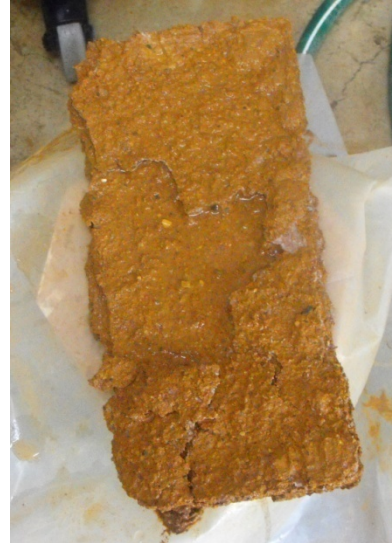
Figure 5.23 and Figure 5.24: Image of results of water pressure test on Panel-3 Earth + Elmer's Glue + Clay, disintegrated fragment after ½ hour continuous water pressure
