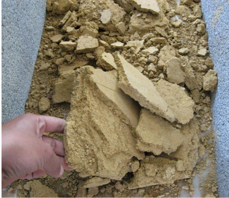
Figure 5.12: Image showing fragmented portions after applying Load test on Panel-5 Earth + Starch
