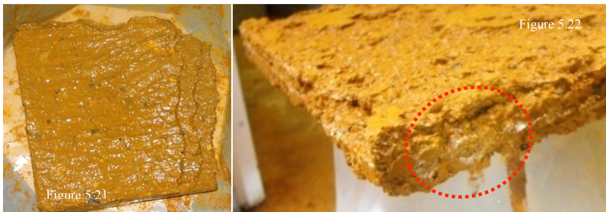
Figure 5.21 and Figure 5.22: Image of results of water pressure test on Panel-3 Earth + Elmer's Glue, disintegrated fragment after ½ hour continuous water pressure
