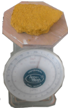
Figure 3.10: Image of Universal Dial Weighing scale (Accu-Weigh) Figure 3.11: Image showing typical loading method used for the research project
