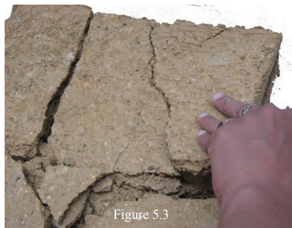
Figure 5.2 and Figure 5.3: Structure of the failed fragments of Panel-6 Earth+ Fly ash
