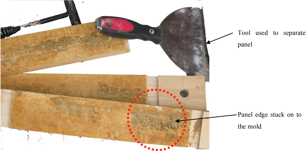
Figure 4.12; Earth stuck on to mold (Panel-3) Earth + Elmer's glue
