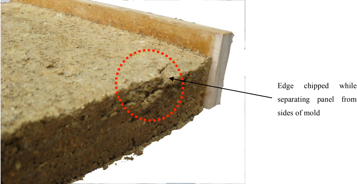
Figure 4.11: Edge detail (Panel-3) Earth + Elmer's glue
