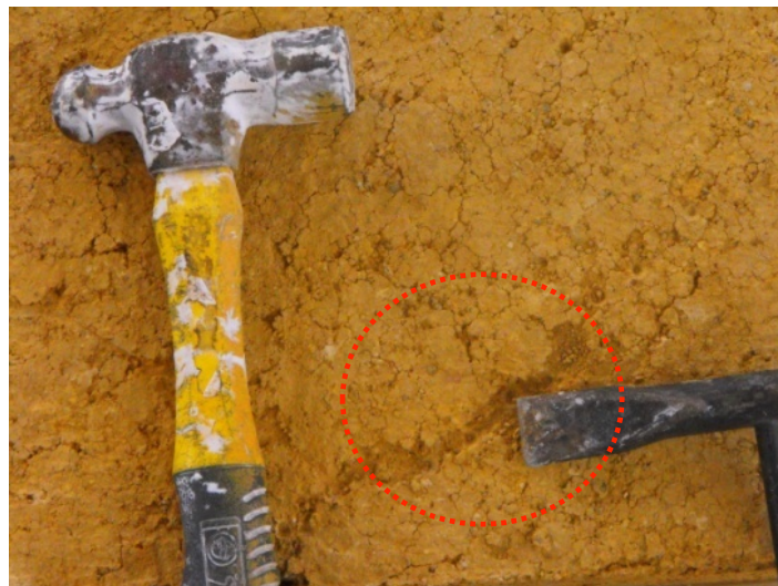
Figure 5.5: Image showing effects of ramming a hammer on the Panel-3 made of Earth + Elmer's glue
