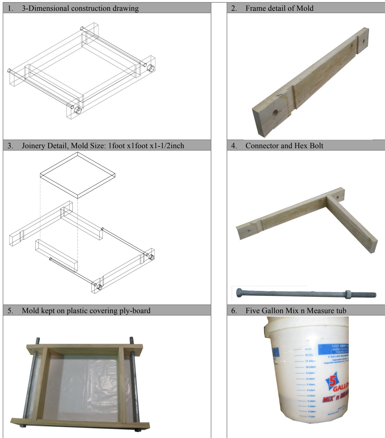
Figure 3.3: Procedure and design of panel mold (Kapfinger, O. 2001)
