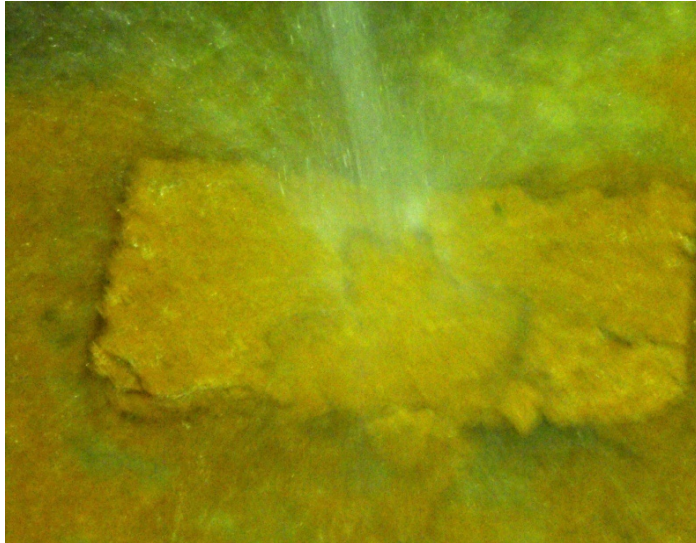
Figure 5.23 and Figure 5.24: Image of results of water pressure test on Panel-3 Earth + Elmer's Glue + Clay, disintegrated fragment after ½ hour continuous water pressure
