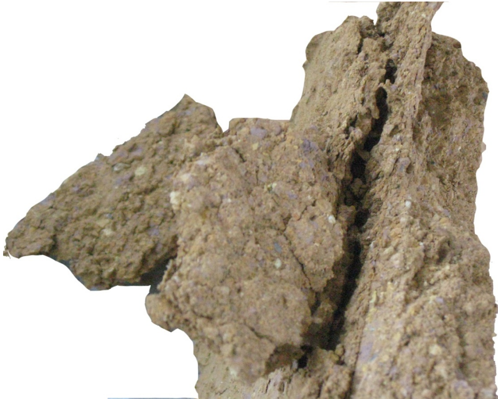
Figure 5.11: Image of fragmented portions after applying Load test on Panel-4 Earth + Clay + Elmer's glue
