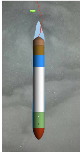
Figure 8.8: Cryobot descending in a pocket of its own melt water.
