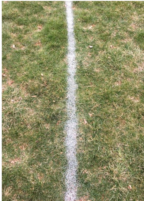
Figure 5.13 Result of Line Painting without the Reference Line
