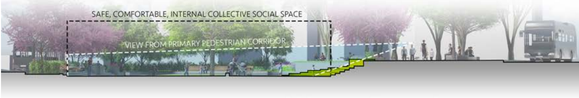
Figure 27 - Utilizing Grade Change To Improve the Quality of the Social Experience. The incorporation of the stepped boundary increases safety for children’s play in the lower collective space while providing views from raised social spaces.
