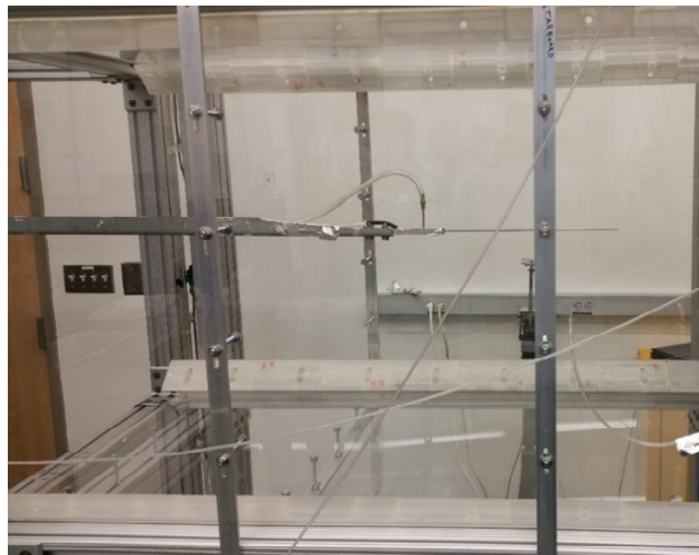
Figure 2.11. The Pitot static probe mounted inside the test section.
