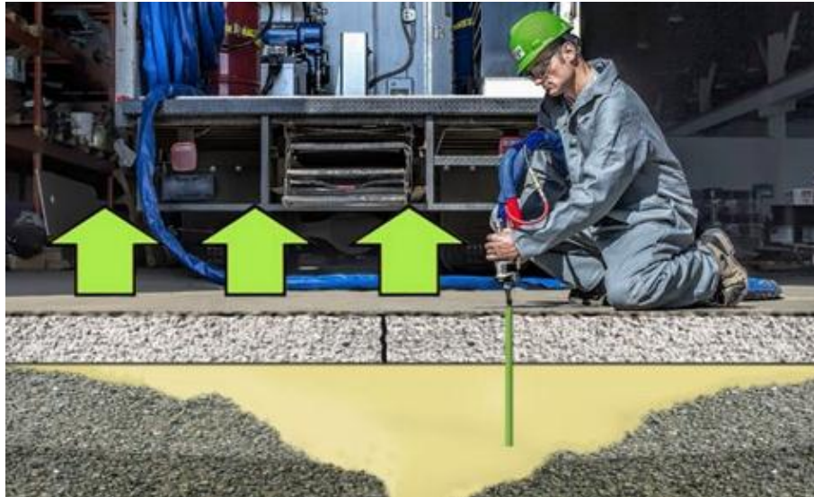
Figure 11: Voids filled with Foam or Grout
