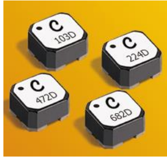
Figure 1.4. LPD 5030V series miniature high-isolation 1:1 two-winding inductor with 1500 V isolation voltage at least occupy 5 \times 5 \text{ mm}^2 footprint and 2.9 mm thickness for an inductance of 4.7 \mu\text{H} [6].
