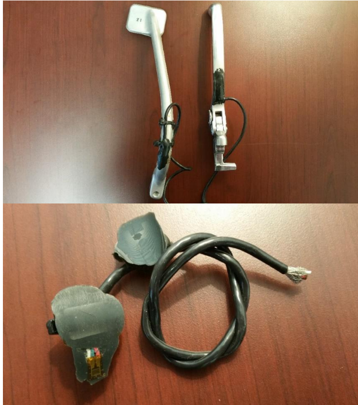
Figure 1. (Top) Strain gauges glued to brake levers, with a rear brake lever on the left and front brake lever on the right. (Bottom) Close-up of the strain gauge surface that is adhered to a brake lever.
