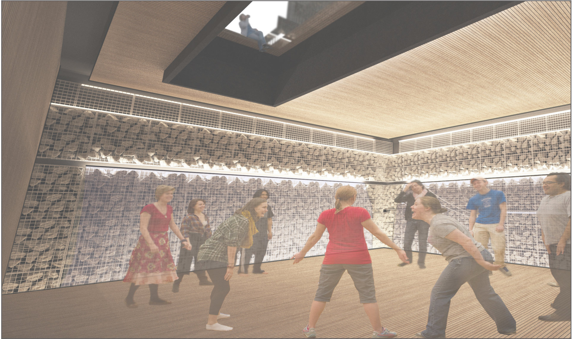
Fig. 8 - rehearsal room featuring water walls with variable acoustic capabilities
