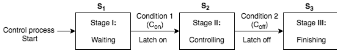
Figure 3.2: Single switch control process
