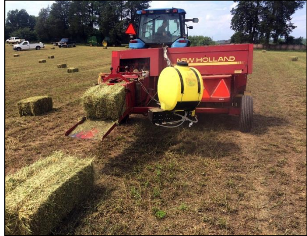
Figure 1. Harvest Tec applicator applying propionic acid at a rate of 2.5 \text{ kg Mg}^{-1} at baling.
