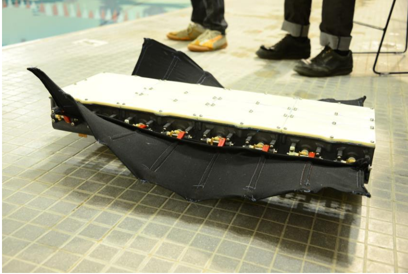
Figure 1-3: A prototype of an undulatory robot developed by CRASH Lab designed to implement fin kinematics similar to those used in the CFD simulations of this manuscript.
