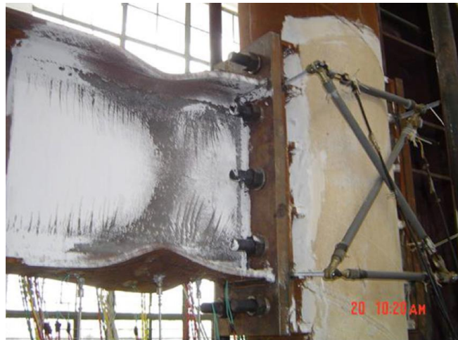
Figure 2-27: Fully cyclic yielding of the RBS with the innovative CCFT connection from test [59]
