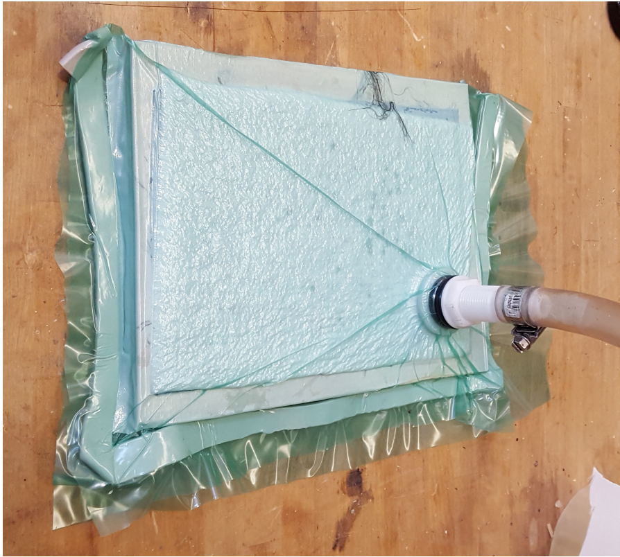
Figure 4.1: Picture of vacuum bagging process on the MFC test article
