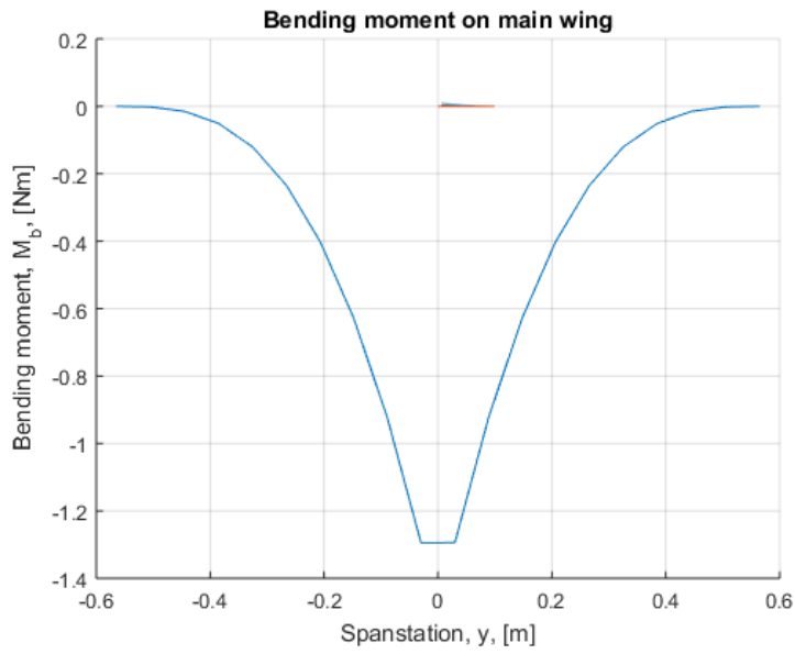
Figure 7.3: Bending moment as a function of span along the main wing of the feathered design.
