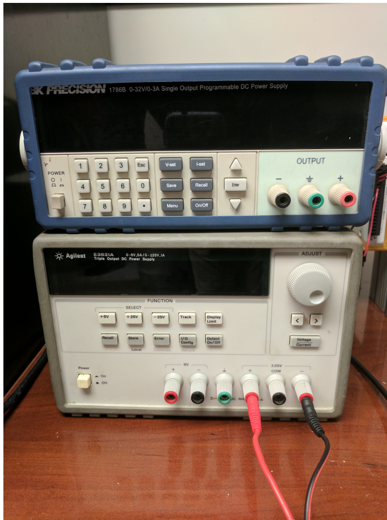
Figure 4.11: Power supplies used for the MFC driver and laser rangefinder
