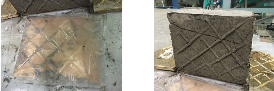
Figure 24 Indented formwork covered with 3.5mil thickness plastic sheet (left). Outcome from trial specimen with this roughening method (right)
