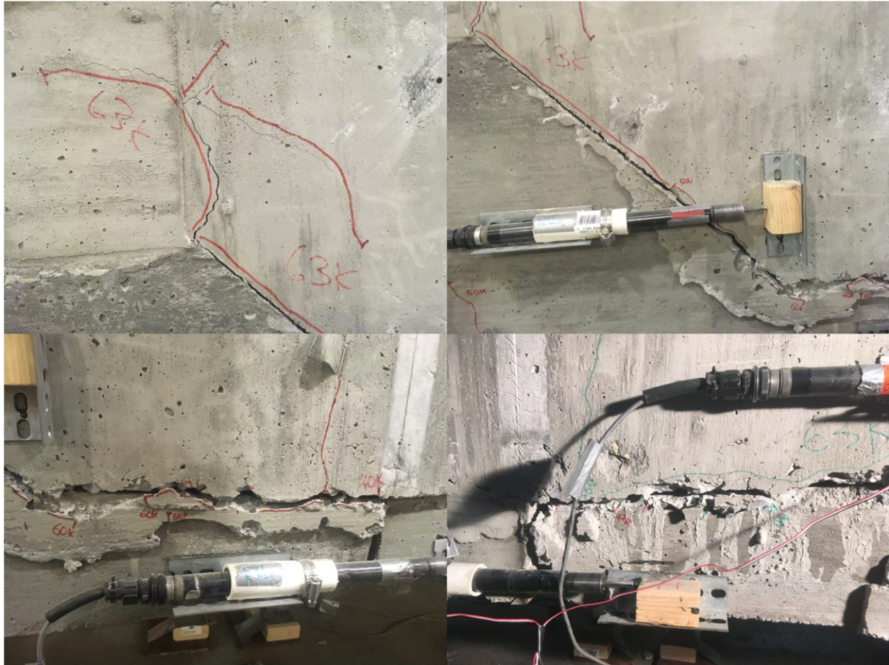
Figure 68 Monotonic load test to failure - cracking at 63 kip actuator load (failure)
