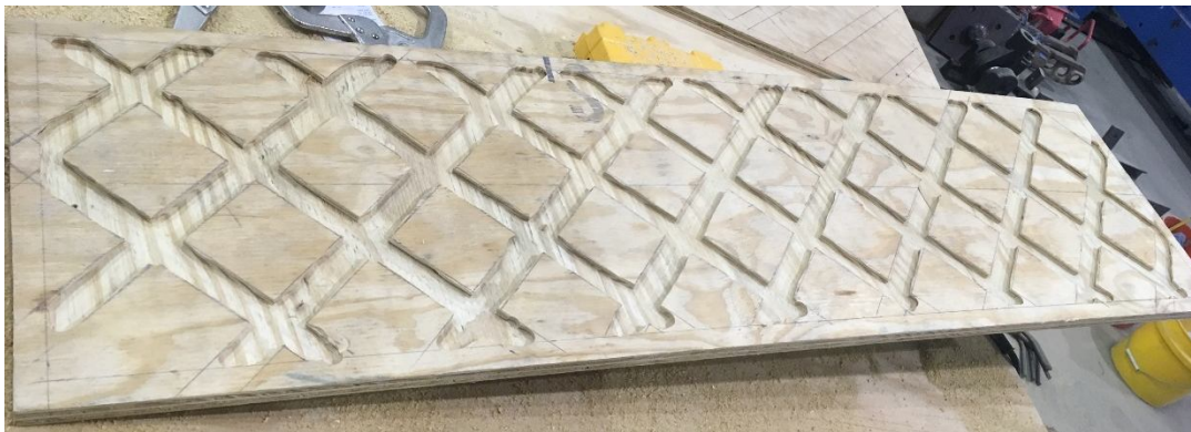
Figure 29 Indented formwork on precast beam flange
