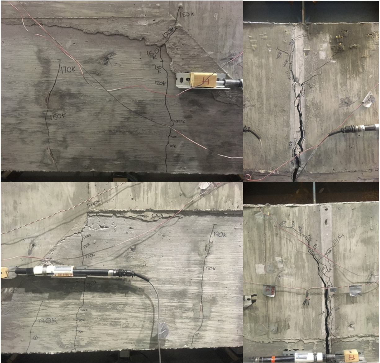
Figure 87 Welded connection specimen failure test - failure at 194 kips
