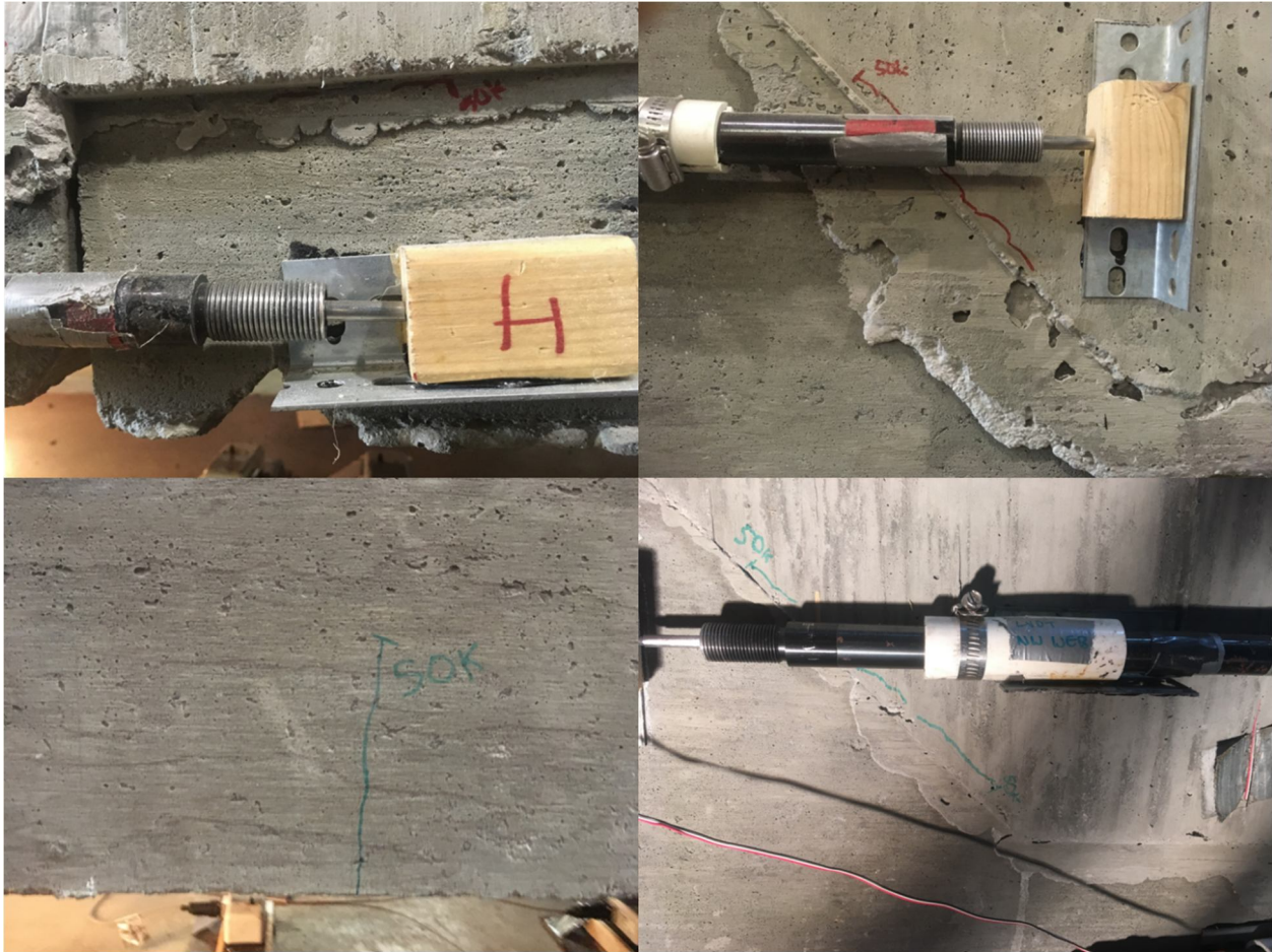
Figure 66 Monotonic load test to failure - cracking at 50 kip actuator load
