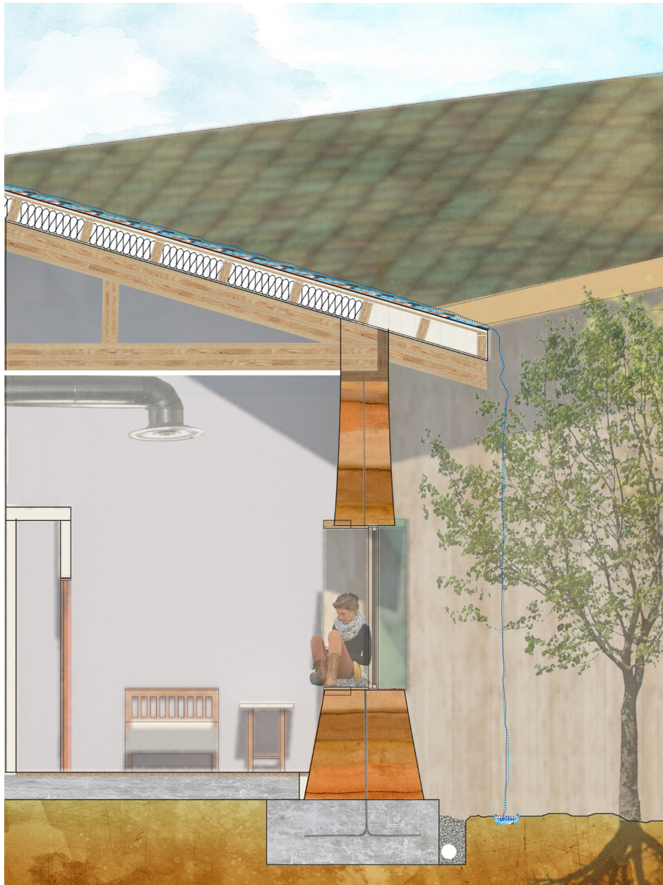
Wall Section with Rainwater
