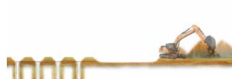
Step 4 Digging for building foundation and vertical loop geothermal pipes, storage of dirt on-site to be used for rammed earth walls (1 month)
