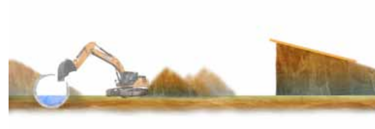
Step 3 Daylighting of creek, soil retained and used as earth sheltering for visitor center (6 months)
