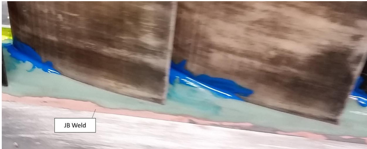
Figure 31. Smooth interface between window and endwall
