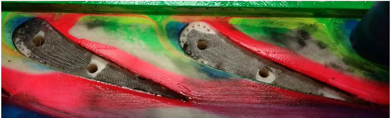
Figure 34. Verification that there is no leakage underneath the vane (underside of vane is also checked)
