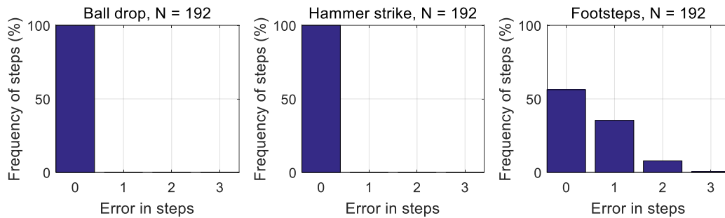
Figure 5.2. Occurrence rate as a function of localization accuracy for the hallway experiment using the custom classification method.
