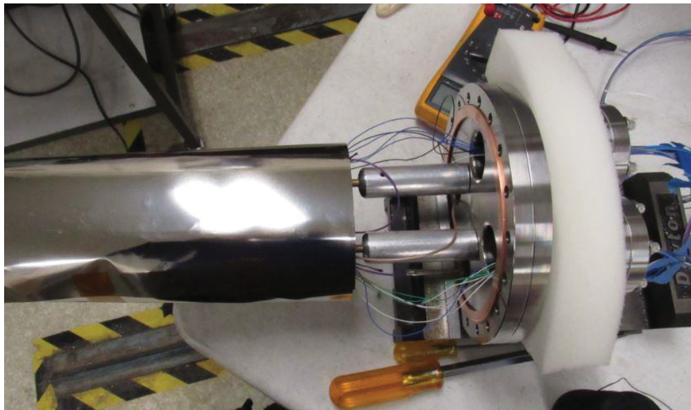
Figure 19b: Outer cylindrical shielding layer for the REDD sensor. Nylon set screws separate the shield from the REDD sensor and mount.
