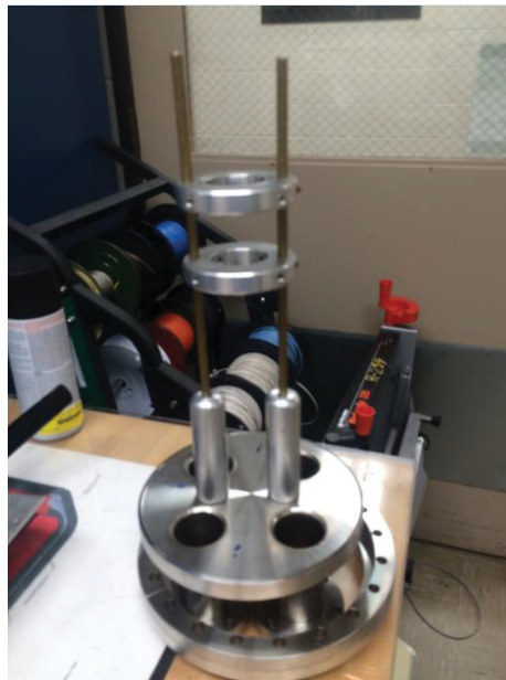
Figure 15: Custom REDD Mount: Magnetically isolated mounting system for positioning and testing of the REDD sensor attaches to the standard 8" CF.
