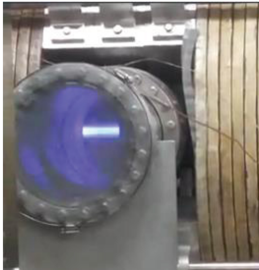
Figure 36: Photograph of a 5eV pulsed AO beam seen during operation of the MSFC AOF.
