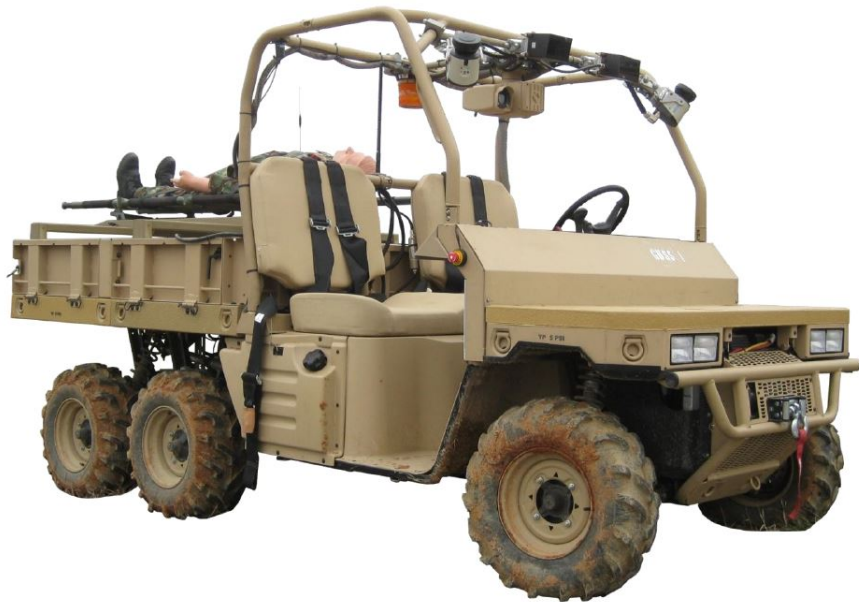
Figure 1.9: GUSS. The LIDAR suite can be seen mounted to the front of the roll cage. Image from [15].
