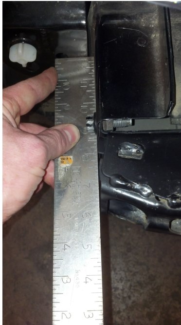
Figure 3.13: Trimmed end of bumper reinforcement.
