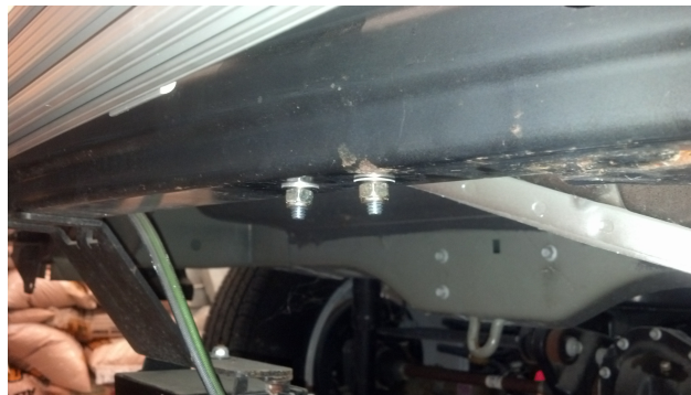
Figure 3.21: Rear bracket bolts go through the rear reinforcement.
