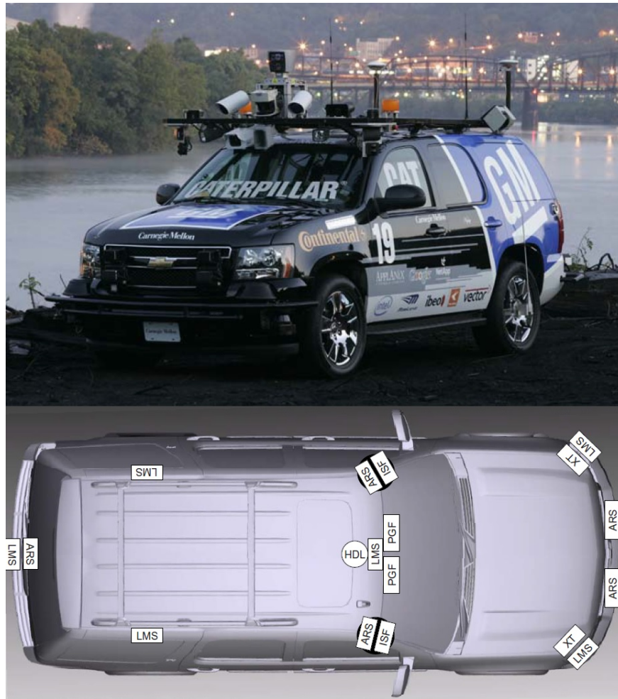
Figure 1.1: Boss and the location of its sensor suite. LMS, HDL, ISF, and XT are LIDARs; ARS is radar; APLX is the GPS/IMU combo; PGF are cameras. Image from [3].
