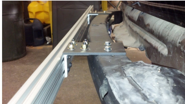
Figure 3.20: Rear bracket supporting rear universal mount.
