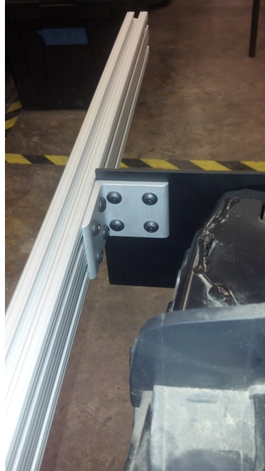
Figure 3.16: Inside view of one bracket mounted to the front passenger side.
