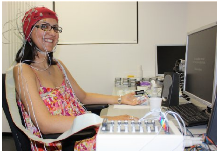
Figure 4.16: The experimental setup for DEAP dataset. The participant seats in front of the a monitor. Video is played on the monitor and the physiological variables are recorded synchronously. image source: www.eecs.qmul.ac.uk/mmv/datasets/deap/ .
