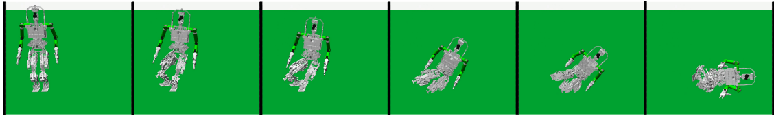
Figure 5.5: ESCHER full degree of freedom lateral fall simulation in ROS Gazebo
