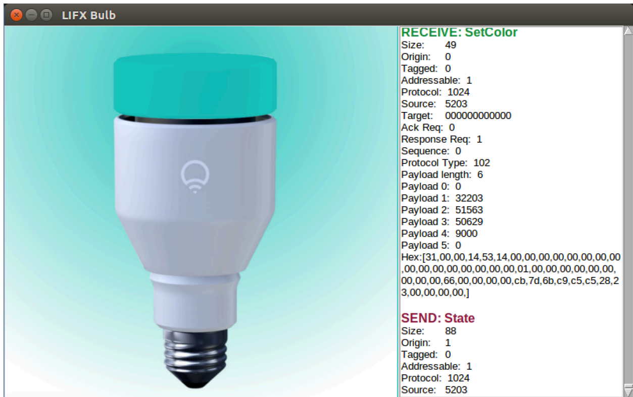
Figure 20. The user interface for bulb_sim.py. It shows a graphical representation of the current lightbulb state and all LIFX messages sent and received by the bulb on the right.
