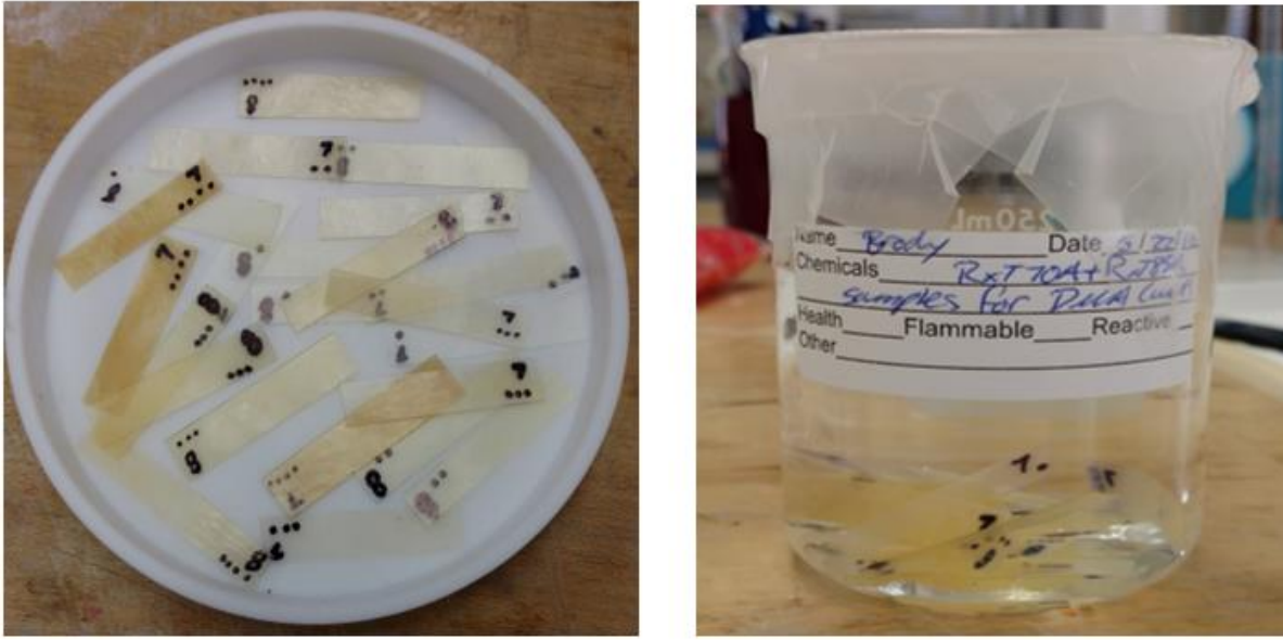
Figure 25. Samples made for DMTA tension testing (dry on the left, wet on the right).
