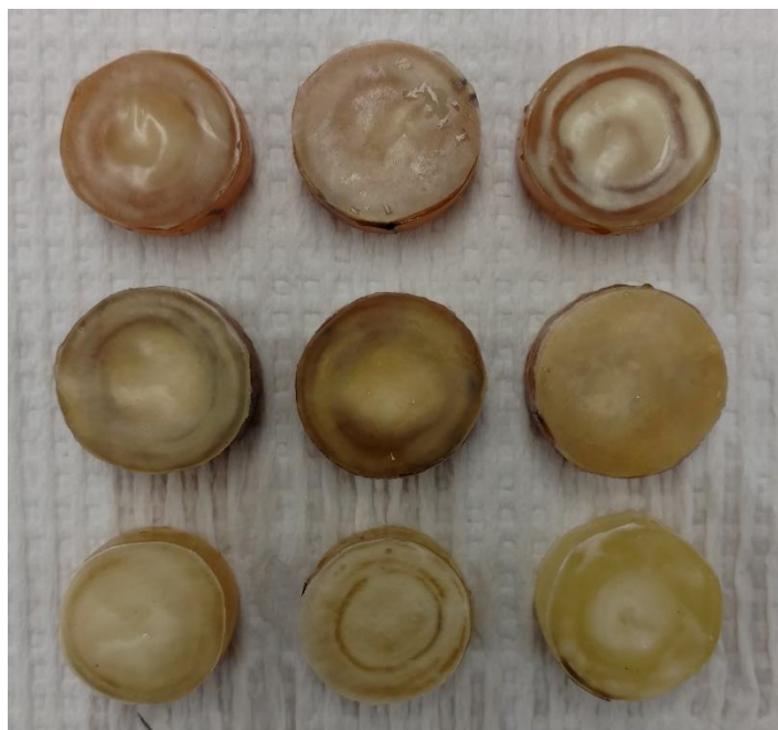
Figure 27. Ringed samples after endplates were attached and middle swelled with water.
