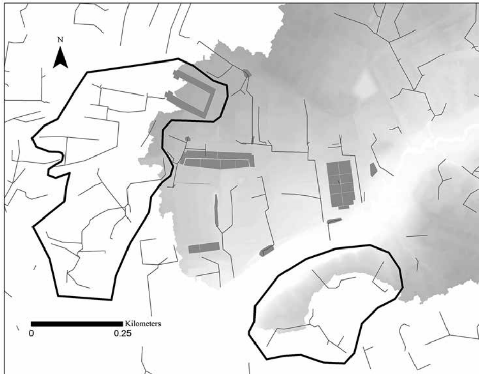
Figure 5. Stormwater network pipes that cross the boundary of the lidar-derived watershed. Dark gray lines and polygons represent stormwater network pipes and facilities. Within the bold black outlines are examples of stormwater pipes and facilities that cross the lidar-watershed delineated boundary.
