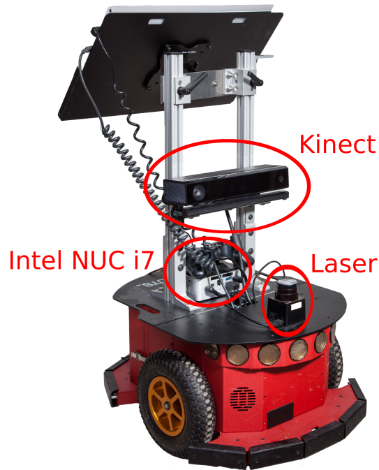
Figure 4.1: Pioneer P3-DX with the onboard Intel NUC i7, Hokuyo laser and Kinect2 sensor used for the experiments. The 2D Hokuyo laser was used for robot localization and the Kinect2 sensor was used for mapping during exploration.
