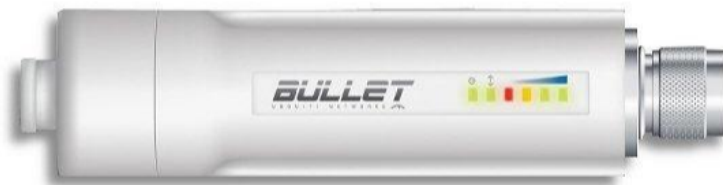
Figure 4.4: Bullet M3 antennas were used to setup global communication.
