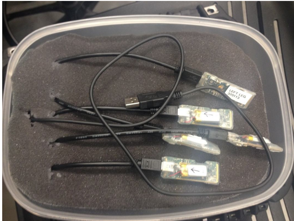
Figure 6: One of two containers set up to organize accelerometers. A USB hub beneath the foam allowed for all accelerometers to be charged and accessed through a single connection to a computer.
