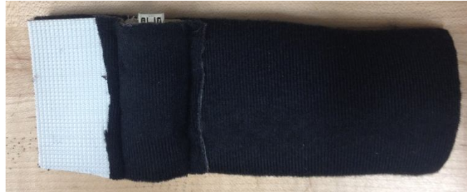
Figure 7: Initial band design featuring an external pouch and section of Velcro hooks for closure.
