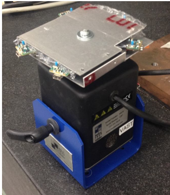
Figure 12: Accelerometers mounted to small shaker for testing.
