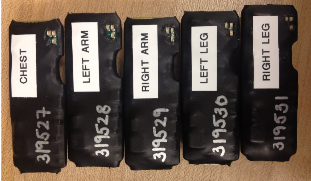
Figure 4: Initial heat shrink wrapped sensors. Use of black heat shrink required holes to be cut for indicator LED's, in the upper right-hand corner, to be seen.
