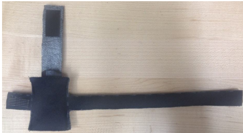
Figure 10: Final band design with flap for sensor cavity open.
