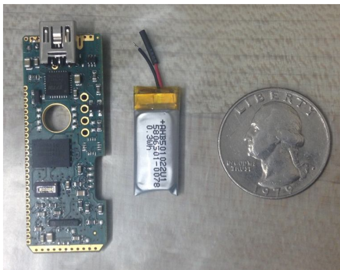
Figure 3: Accelerometer circuit board shown with replacement battery and quarter for size reference.
