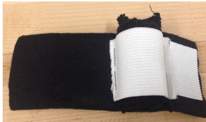
Figure 8: An iteration of the band design, including an elastic material to form a pocket.
