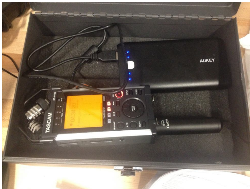
Figure 14: Recorder, external microphone, and external battery placed in lock box, as intended during data collection.
