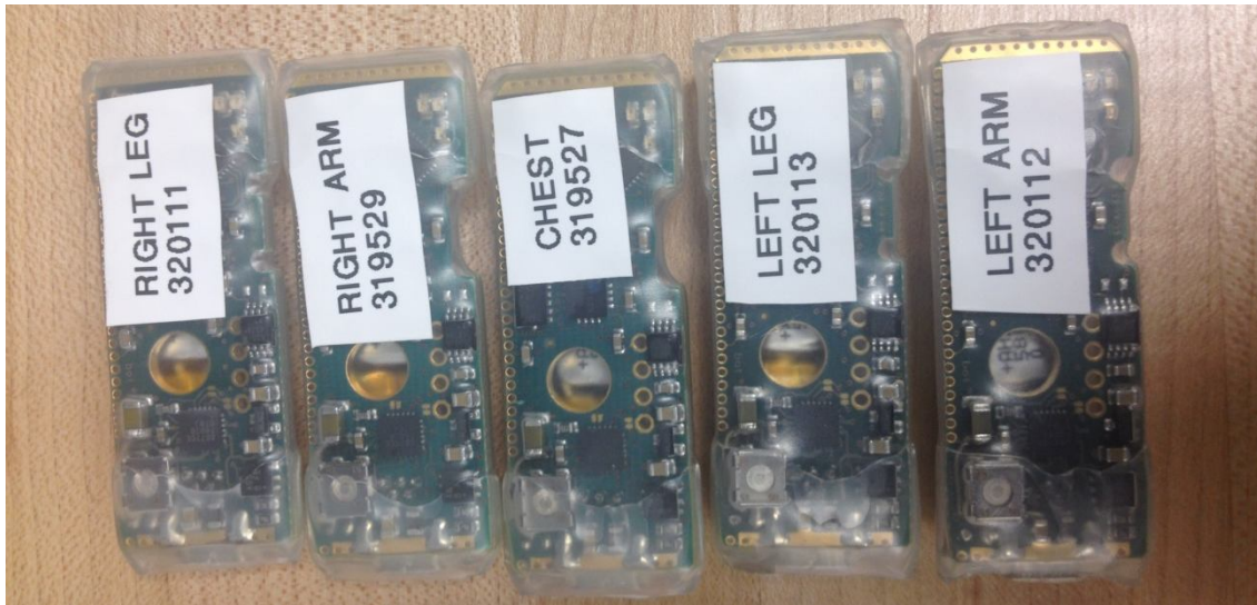
Figure 5: Re-enclosed sensors, wrapped in clear heat shrink to improve seal and allow LED's to be seen without holes.
