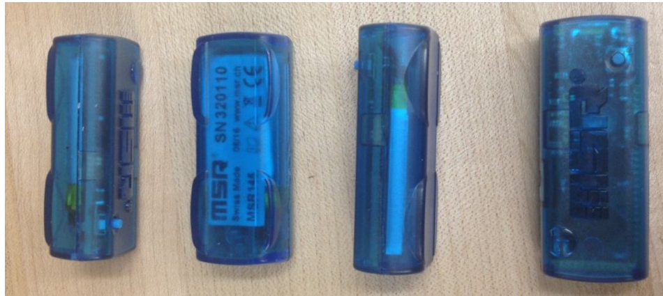
Figure 2: Modular Signal Recorder (MSR) 145 3-axis accelerometers purchased for use on this project.
