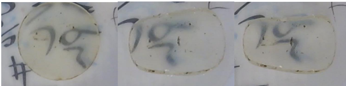
Figure 4.1: 60 wt % CNC film before water was added (left), 15 minutes after water was added (center), and one hour after water was added.
