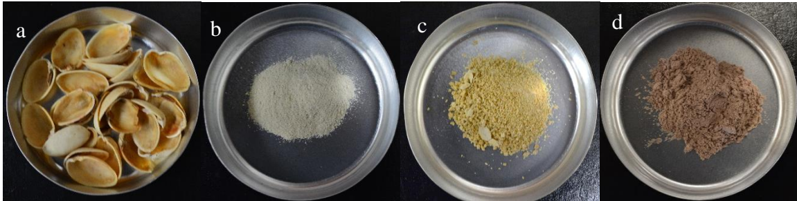
Figure 3.1a: Pistachio in the shell. b: Milled shell. c: Post extraction cellulose. d: Dried CNCs.
