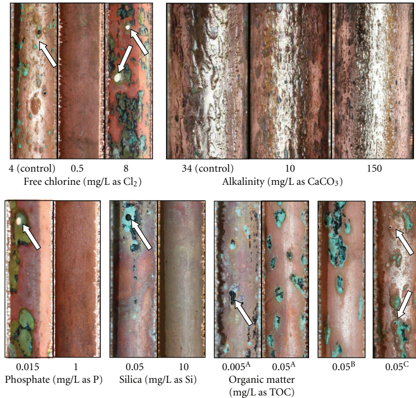
FIGURE 3: Representative photographs of copper from selected tests following scale removal. Photos are grouped by respective adjustments to control water quality ( A NOM, B ozonated NOM, C sodium acetate/d-glucose), and arrows indicate some of the pinhole leaks that formed during testing. All photos show copper from small-scale tests, except for those in the variable alkalinity group.
