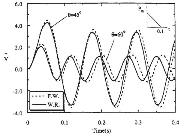
Fig. 5. Influence of the warping restraint and of the ply-angle orientation on time-history of the dimensionless deflection of the beam tip; blast pulse,  $t_p = 0.1$  s,  $r = 1$ ,  $AR = 16$ , non-shearable beam model.
