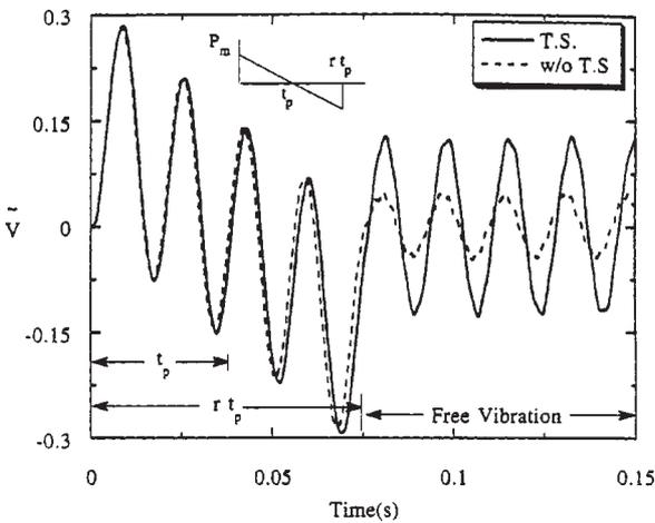
Fig. 4. Influence of transverse shear on time-history of the dimensionless deflection of the beam tip, sonic boom pulse,  $t_p = 0.037$  s,  $r = 2$ ,  $\theta = 45^\circ$ ,  $AR = 6$ , free warping model (FW).
