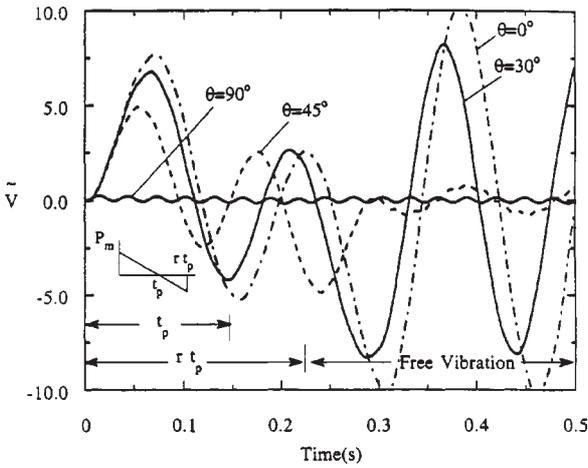
Fig. 3. Influence of ply-angle on time-history of the dimensionless deflection of the beam tip. Sonic-boom overpressure signature.  $t_p = 0.15$  s,  $r = 1.5$ ,  $AR = 16$ ; non-shearable and free-warping beam model.
