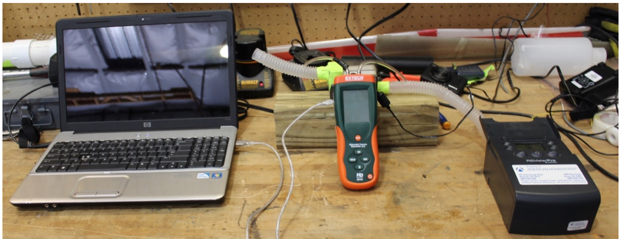
Figure 21. The industry-produced intake bacterial filter testing for comparison to prototype filters.
