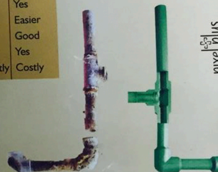
GI Pipes After 10 Years
