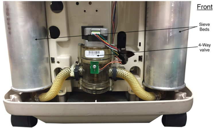
Figure 12. Internal components in the front of the oxygen concentrator [2].
