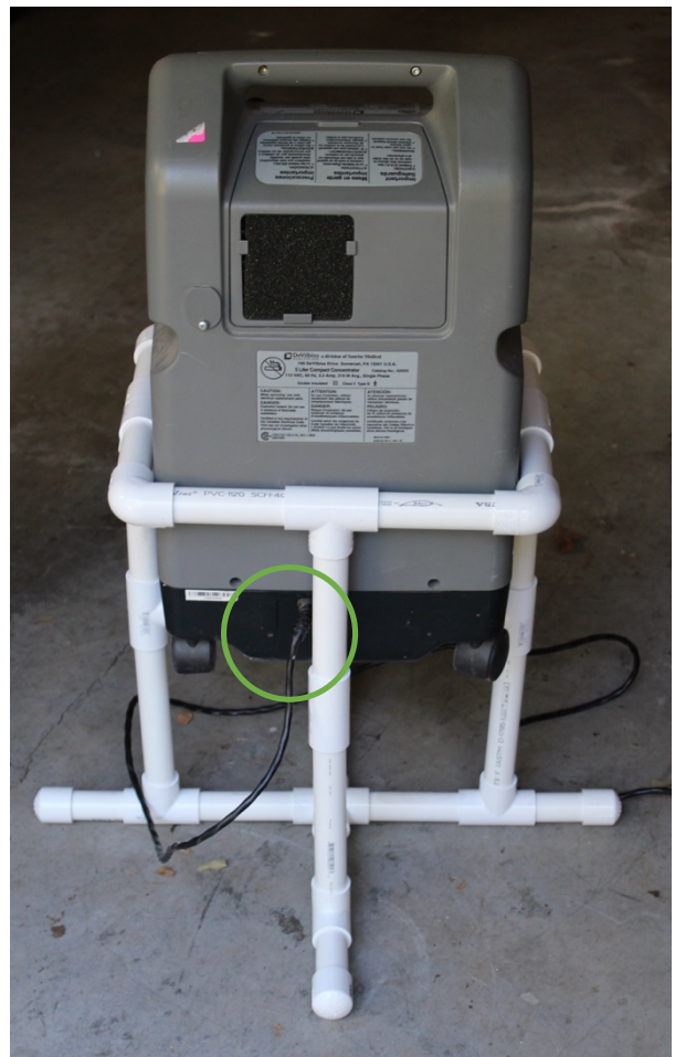
Figure 32. The oxygen concentrator in the ventilating stand, with the cord protruding left of the center support.
