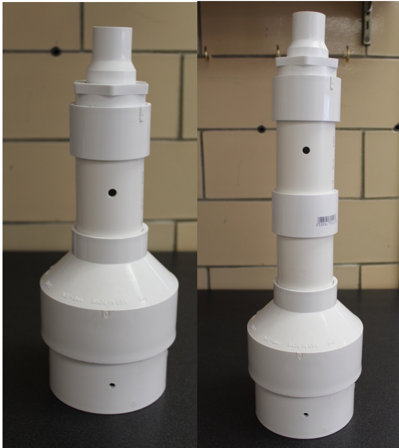
Figure 23. The single-layer (left) and depth capsule (right) devices for bacteria projection onto a petri dish.
