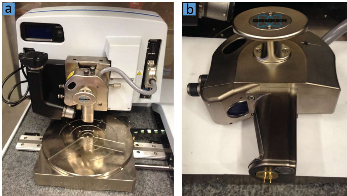
Fig. 6.2. Photos of Bruker Dimension Icon AFM and its scanning head.
