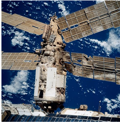
Figure 1.7: Damage to Mir seen from Atlantis during STS-86, credit: NASA
