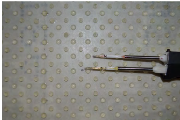
Figure 5.5: Parallel quadwires (top left) and vertically aligned single hotwire (top probe of right picture) and flattened Pitot (bottom probe of right picture) measuring velocity on mixed-shape rough surface (flow moving left to right)
