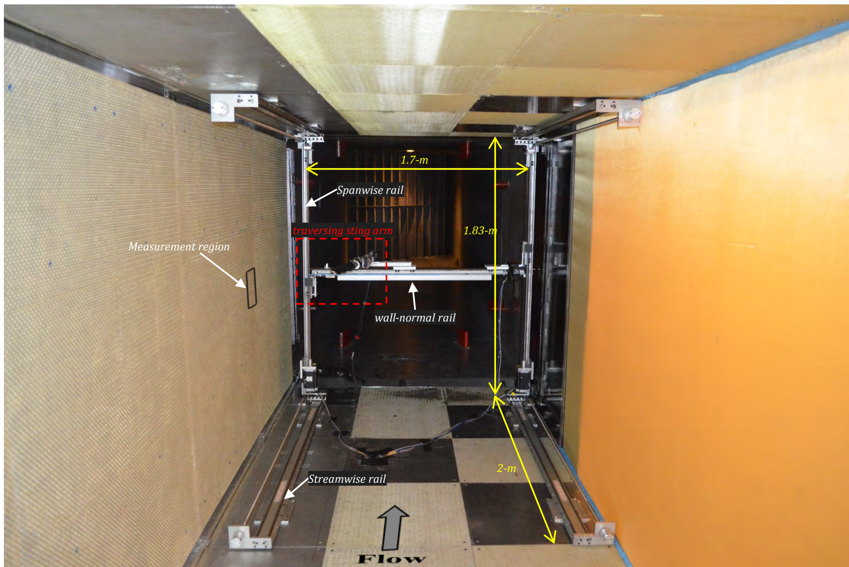
Figure 2.16: Upstream view looking downstream at the three-axis traverse system installed in the test section of the Stability Wind Tunnel
