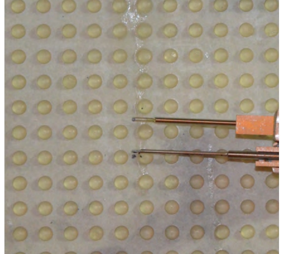
Figure 5.2: Vertically aligned quadwires (left) and vertically aligned single hotwire (top probe of right picture) and flattened Pitot (bottom probe of right picture) measuring velocity on intermediate rough surface (flow moving left to right)
