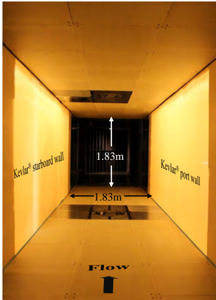
Figure 2.2: Upstream view looking downstream of the anechoic test section of the Virginia Tech Stability Wind Tunnel
