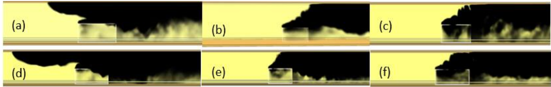
Figure 8.3. The effect of different velocities on smoke propagation of 10 MW and 30 MW vehicle fires in the road tunnel at t=100 s (a) 10 MW, 1.5 m/s (b) 10 MW, 2.8 m/s (c) 10 MW, 5 m/s (d) 30 MW, 1.5 m/s (e) 30 MW, 3.7 m/s (f) 30 MW, 5 m/s
