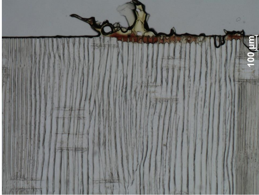
Figure 6-9: Example penetration of PLY RESIN on loblolly pine; 5X (n =13-29 cells per slide with n = 10 slides)
