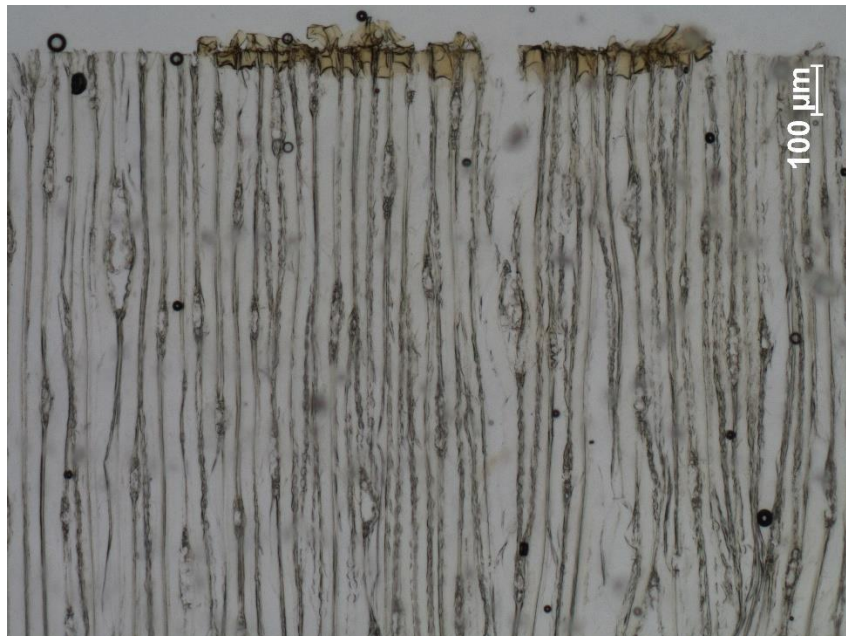
Figure 6-8: Example penetration of PLY RESIN on loblolly pine; 5X (n =13-29 cells per slide with n = 10 slides)
