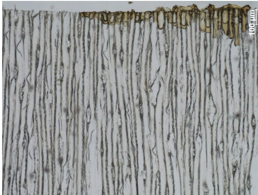
Figure 6-7: Example penetration of PLY RESIN on loblolly pine; 5X (n =13-29 cells per slide with n = 10 slides)
