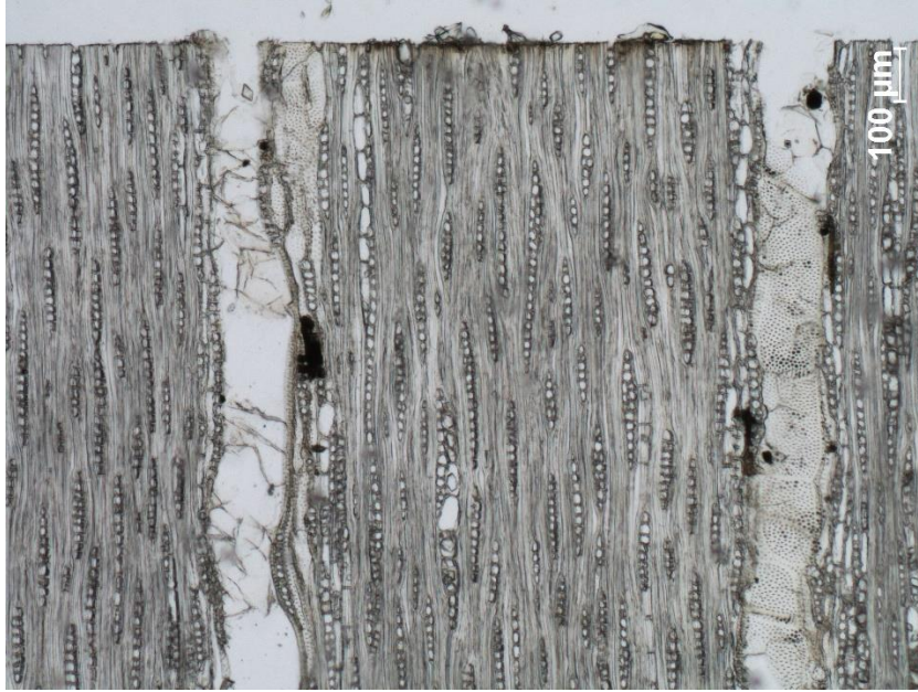
Figure 6-15: Example penetration of PLY SURF 0.5% on spotted gum; 10X (n =19-66 cells per slide with n = 10 slides)
