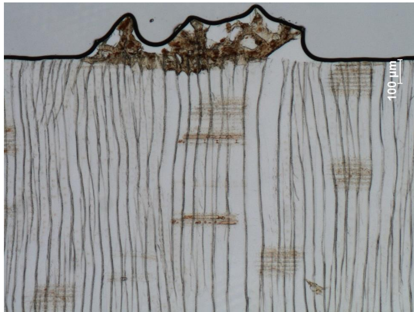
Figure 6-12: Example penetration of PLY FORM on Douglas-fir; 5X (n =16-24 cells per slide with n = 9 slides)
