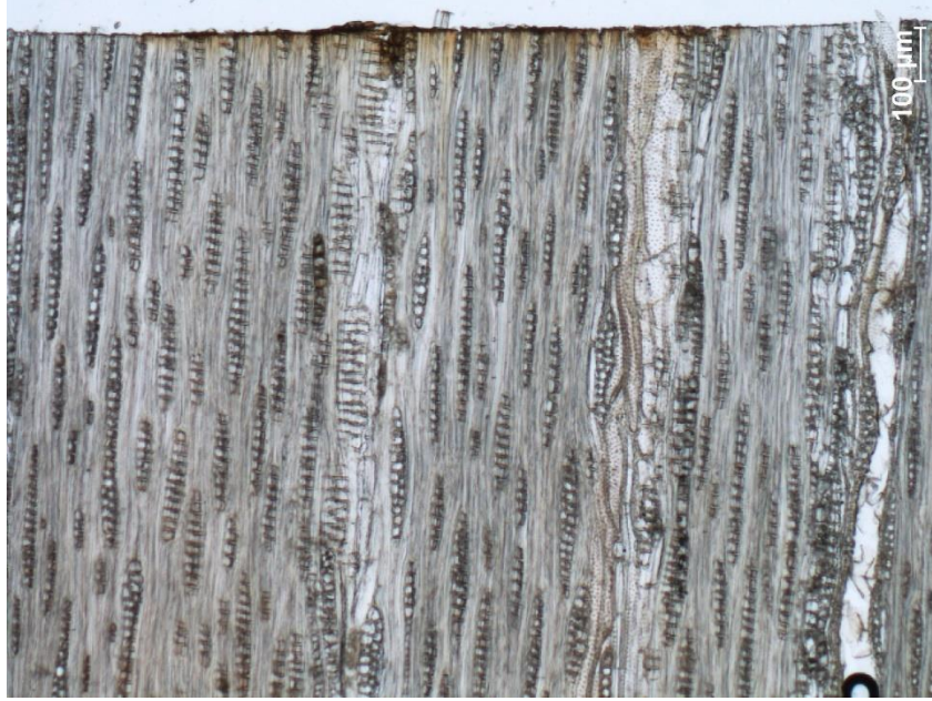
Figure 6-13: Example penetration of PLY SURF 0.5% on spotted gum; 10X (n =19-66 cells per slide with n = 10 slides)
