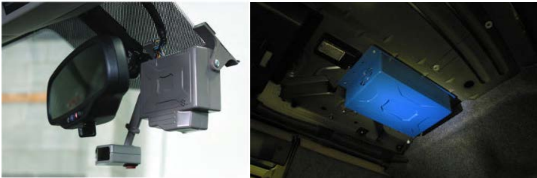
Figure 2. Photos. SHRP 2 DAS installation: head unit behind rearview mirror (left); main unit onto the roof of the vehicle's trunk (right).
